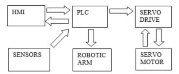
Fig. 1 System Block Diagram
